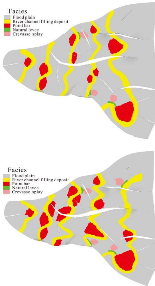
Figure 5: Sedimentary facies model map of Ed3III-8 sublayer in the study area: (a) Sedimentary facies model based on two-dimensional training image; (b) Sedimentary facies model based on three-dimensional training image.
