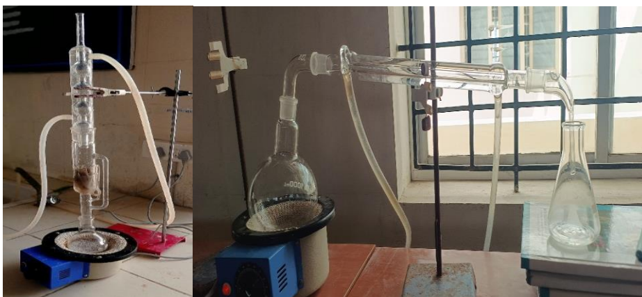
Figure 3: Experimental setup of Soxhlet extraction (left) and simple distillation unit (right) used for isolating and concentrating biopesticidal compounds from Annona squamosa seed extract.
